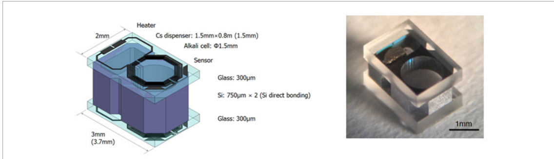
Figure III-2 Fabricated MEMS Vapor Cell Structure and Photograph
